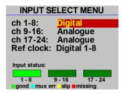
the main screen will indicate when the Reference clock is missing or when a digital signal slip occurs. Reference clock (see below) can also be set in this menu screen.
