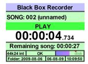
If the BBR is set to "PLAYBACK LOCKOUT" and you want to disable it temporarily to perform a Virtual Sound Check, press the MENU button to enter the MENU and PLAYBACK LOCKOUT is the first item on the list. Press MENU again and it will remove the tick ( ) mark against PLAYBACK LOCKOUT. Press BACK to exit the MENU and you can now use Playback normally. PLAYBACK LOCKOUT can be set to manual in the SETUP menu preventing it automatically engaging after each recording
