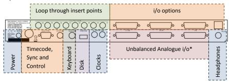
The lower 3 D-type (sometimes called D-sub) connectors\* are the main unbalanced analogue i/o connectors on the BBR1U, BBR1A and BBR1D. The cable looms conform to the TASCAM standard for analogue i/o (N.B. all pin outs are available on the visitor page of the JoeCo website Login area)
