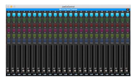
The Mic/line Input control window allows control of the BBWR's Inputs and effects. When Mic is selected the +48V (phantom power), HPF (High Pass Filter), Limit (soft limiter), 28dB Pad and Phase reverse buttons become active. The green Limit buttons turn amber to indicate that the limiter has been activated to reduce the level on that channel. Faders adjust the input level gain and you can also type accurate gains into the field at the bottom of each fader.
