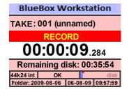
press the REC button again. You can also set MARKS by pressing the MARK button which will appear in the Cue Chunk of the BWAV files which some DAWs can use and will enable you to create loops easily for Virtual Sound Checking.
