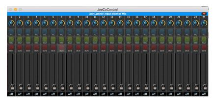
The Low Latency Input Monitor Mix window allows control of the local Low Latency headphone Monitor Mix on the BlueBox providing Pan and Level controls for each channel of the monitor mix along with familiar mute and solo functions. The resultant mix is routed to the rear headphone socket and is available for a producer or director to listen to the monitor mix during the recording.
