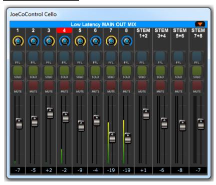
There are up to 4 low latency monitor mixes available depending on your operating mode – MAIN (monitor mix), ph 1 (headphone mix 1), ph2 (headphones 2), digital (not available at higher sample rates). These mixes allow you to create discrete low latency monitor mixes for monitoring or foldback purposes.
