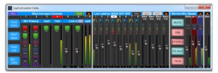
The first (left hand) section is the input controls and master settings panel.
